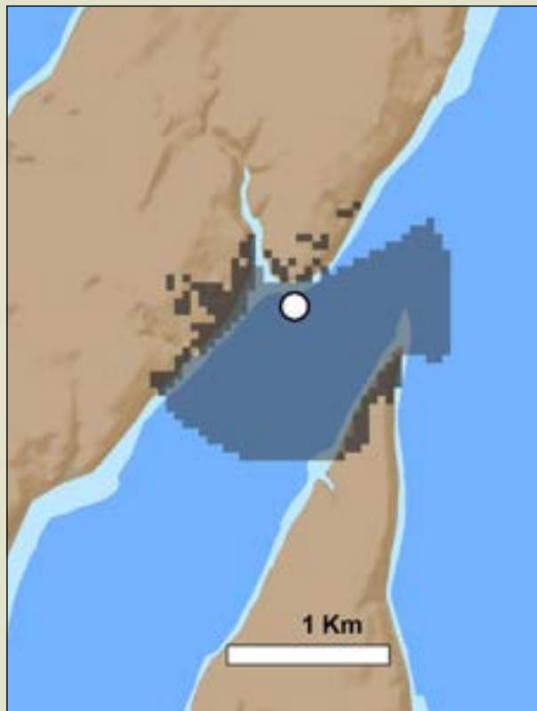
An example calculation of the area from which a proposed farm structure (open circle symbol) may be visible using the Scenic Quality tool (Tallis et al. 2013). The dark shading surrounding open symbol corresponds to areas from which the site may be visible.
